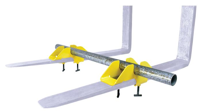
The SMP-FLA-4 forklift attachment is ideal for lifting, transporting or payout of materials stored on a reel. The heavy-duty T-Handle locking mechanism ensures this reel roller will hold steady regardless of pull strength or forklift driver. Designed to work with 4" wide forks, the SMP-FLA-4 attachment (sold in pairs) features 1/4" laser-cut steel construction with a powder coated finish, and a 48" arbor support bar that must be used to support the reel.
