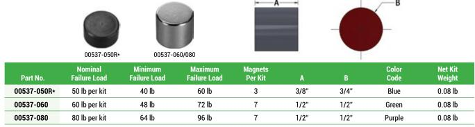
Note: The magnets are designed to separate within +/- 20% of their nominal failure load.
