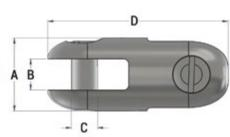
The two smaller sizes have slotted clevis pins, while the larger sizes have hexagon clevis pins, all of which are available as spares (see page 11).
