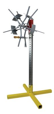
Ideal for re-coiling materials stored on a reel rack system, the SMP-CR-12 height adjustable coiler forms a 12" inside diameter round coil which can be tied before collapsing. Unlike most other coilers on the market, the SMP-CR-12 offers a smoother collapse that can be performed single-handedly with ease by any operator. When collapsed, the formed coil off-loads to the front of the machine. This collapsible coiler features a heavy-duty welded steel base with telescopic upright section.
