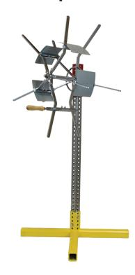
Ideal for re-coiling materials stored on a reel rack system, the SMP-CR-16 height adjustable coiler forms a 15" inside diameter round coil which can be tied before collapsing. Unlike most other coilers on the market, the SMP-CR-16 offers a smoother collapse that can be performed single-handedly with ease by any operator. When collapsed, the formed coil off-loads to the front of the machine. This collapsible coiler features a heavy-duty welded steel base with telescopic upright section.
