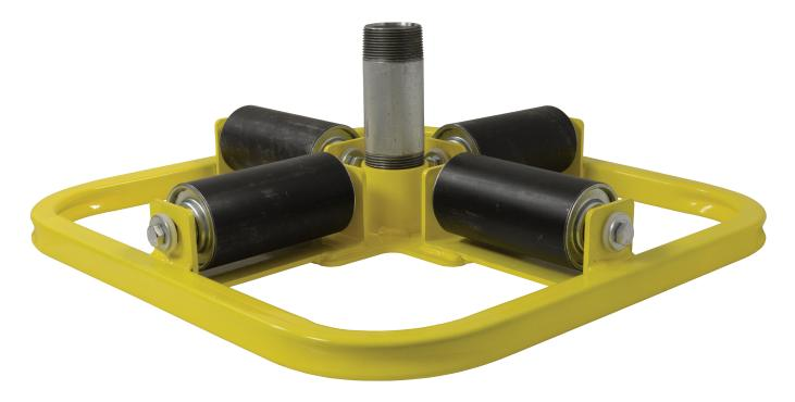
The SMP-CS series of industrial lazy susan turntables are engineered for horizontal pay out of wire, cable or other material stored on reels. The SMP-CS-24 reel turntable is ideal for cable reels with flange or arbor hole damage. The SMP-CS-24 is designed to support reels up to 1,000 lbs and comes standard with a 2" arbor spindle for fast set-up and operation.
