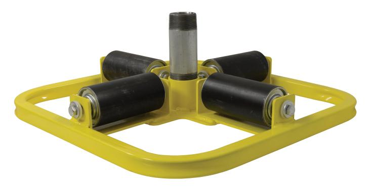
The SMP-CS series of industrial lazy susan turntables are engineered for horizontal pay out of wire, cable or other material stored on reels. The SMP-CS-48 reel turntable is ideal for cable reels with flange or arbor hole damage. The SMP-CS-48 is designed to support reels up to 3,000 lbs and comes standard with a 2" arbor spindle for fast set-up and operation.
