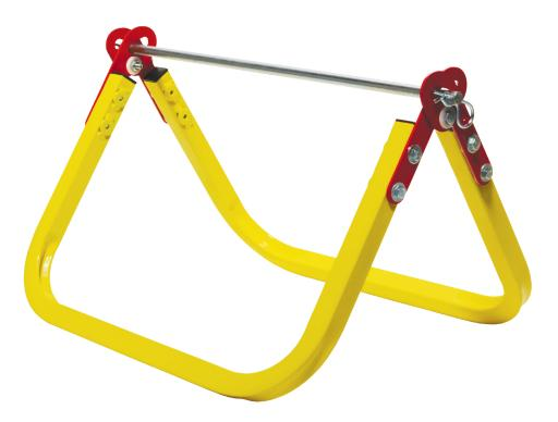
This versatile and rugged folding wire caddy is designed for years of reliable in-field service. Constructed from welded steel tubing, the SMP-DC-1 caddy features one (1) 0.5" diameter solid steel zinc-plated spool support bars and a durable powder coated finish. The unique folding mechanism facilitates convenient transport and storage. The SMP-DC-1 will hold one (1) spool up to 16.5" wide x 20" diameter with a weight capacity of up to 100 lbs.
