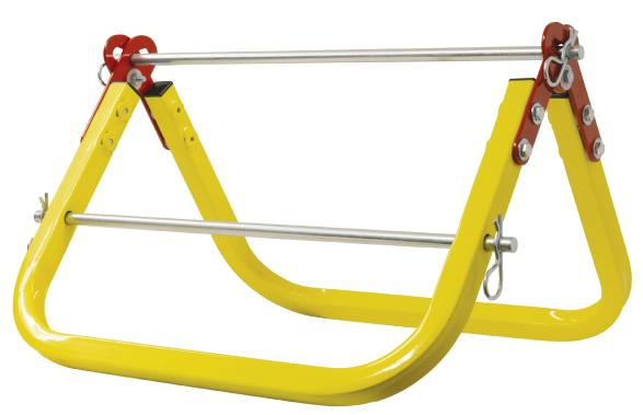
This versatile and rugged folding wire caddy is designed for years of reliable in-field service. Constructed from welded steel tubing, the SMP-EC-4 caddy features two (2) 0.5" diameter solid steel zinc-plated spool support bars and a durable powder coated finish. The unique folding mechanism facilitates convenient transport and storage. The SMP-EC-4 will hold one (1) spool up to 16.5" wide x 20" diameter or four (4) spools up to 8" wide x 8" diameter.
