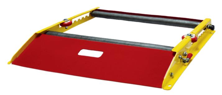
The SMP-RP-27HD reel roller system is ideal for storage, dispensing and management solutions of cable reels ranging from 12" to 48" in diameter. The SMP-RP-27HD can accommodate cable drums up to 27" wide with weights up to 3,000 pounds. The seven (7) gauge steel frames include six (6) position adjustments for the rollers, a slanted loading ramp, front roller locks for easy loading & unloading, and pre-drilled holes for permanent mounting applications.
