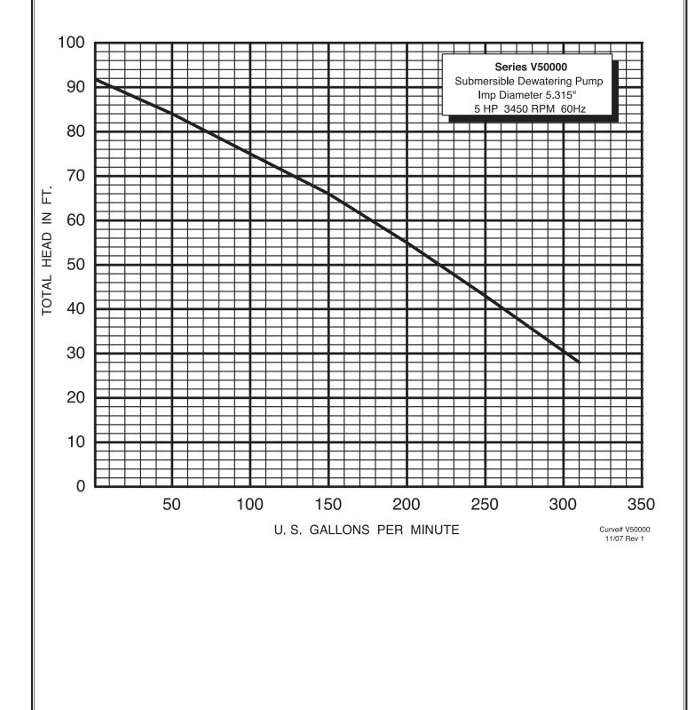
Submersible Dewatering Pumps 3" NPT Female Discharge
